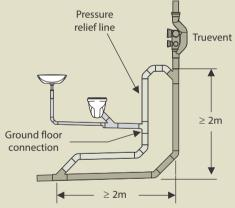
3. A typical installation of single stack system with Truevent aerator.
