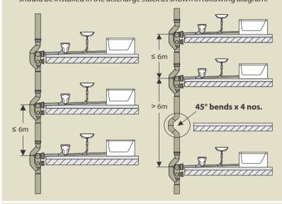
2. To eliminate the possibility of pressure build up in single stack system, it is recommended to provide the pressure relief line of 110mm size as given below:-
